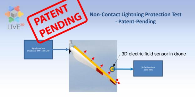
The electic field is always upright to metal. This fact enables the analysis of direction and intensity of the electric field and can prove the existance of an intact earth connection savely.
