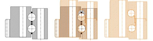
T-Solid (in orange color) compared with 4-point contact pitch bearing to be replaced – same bolt pattern, same gearing! Longer bolts are required due to slightly increased bearing height.
