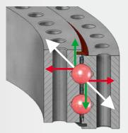
In 4-point contact pitch bearings the forces always result in radial loads which periodically widen the outer bearing rings.
