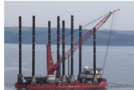
d) Jackup barge
