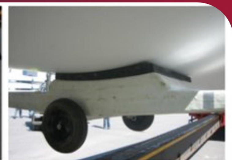
Figure 12-5: Saddle and lifting shell placed under the blade
